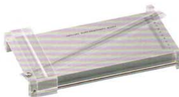
Standard percentage reader (aluminum) for rotor HT-24
